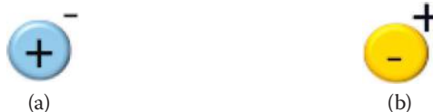
FIGURE 8.14 (a) Fixed positive charge and free negative charge; (b) fixed negative charge and free positive one.
