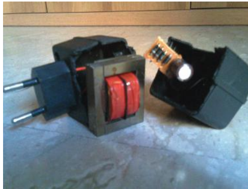
FIGURE 9.17 A common power supply inside of its box: we can clearly see the transformer (with the red cable coils), the four diodes (that form the Graetz bridge), and the capacitor.
