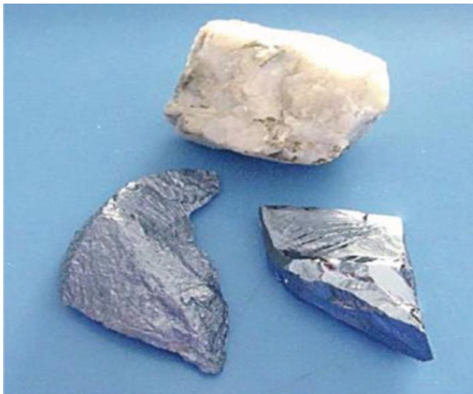
FIGURE 3.29 Silicon dioxide compound ( \text{SiO}_2 ) (top), intrinsic silicon ( \text{Si} ) (bottom).
