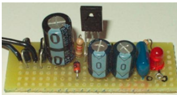
FIGURE 9.15 Simple stabilized power supply made by students of the course “Laboratory of Electronics” held at University of Rome Tor Vergata.
