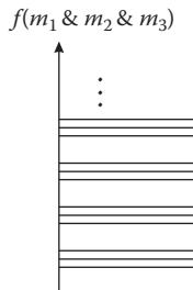
FIGURE 3.17 Split frequencies for a system of three coupled oscillators.
