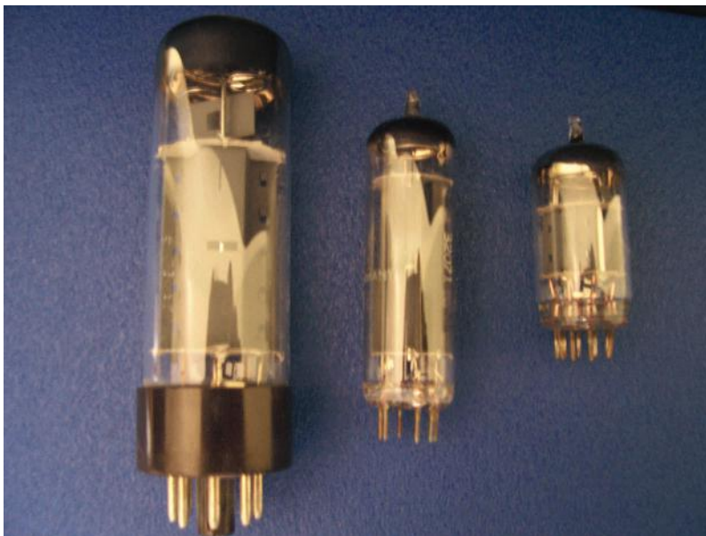
FIGURE 8.38 Valves. Once they performed the tasks assigned today to transistors.
