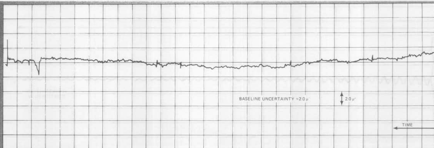
Fig. 12—A 20 nW pulse released 1 in. from the monitoring sensor into the oven described in Fig 11 produced this extraordinary trace. Peak temperature rise is 7 microdegrees.
