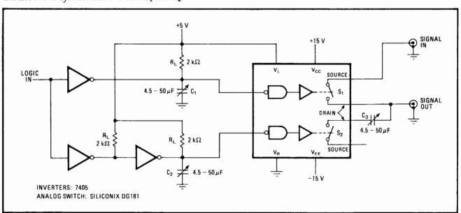
**Squelching spikes.** Switching transients at the output of an analog FET switch can be greatly attenuated by synchronizing the turn-on and turn-off of one switch with those of a second switch. Open-collector TTL inverters produce logic pulses whose output rise times can be varied while their output fall times remain fixed. The turn-on of switch  $S_1$  is made to coincide with the turn-off of switch  $S_2$ , and vice versa.
