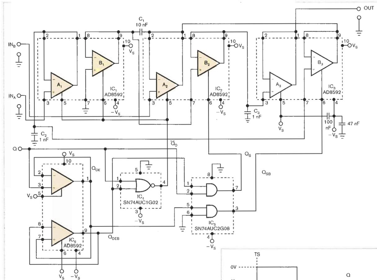
Figure 1 The basis for the operation of this circuit is the simultaneous tracking of the  $V_{IN_A}$  and  $V_{IN_B}$  input voltages on capacitors  $C_1$  and  $C_2$  and a stacking of these capacitors within the sample interval on capacitor  $C_3$ .
