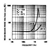
Eliminating zeners reduces typical high frequency noise by nearly a factor or 10. Worst case noise is reduced even more. High frequency noise of LM102 has caused problems when it was included inside feedback loop with other IC op amps.
