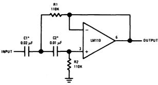
\*Values are for 100 Hz cutoff. Use metalized polycarbonate capacitors for good temperature stability TL/H/8462-4
