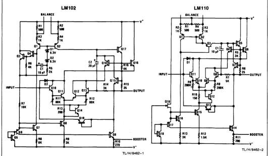
Biggest design difference between the LM102 and LM110 is the elmination of the zener diodes (D1 and D2) in the biasing circuit. This reduces noise and permits operation at low supply voltages.
