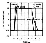
TL/H/8462–3 Large signal pulse response shows 40V/ $\mu$ s slew for LM110 and 10V/ $\mu$ s for LM102. Leading edge overshoot on LM110 is virtually eliminated, so external clamp diode frequently required on the LM102 is not needed.
