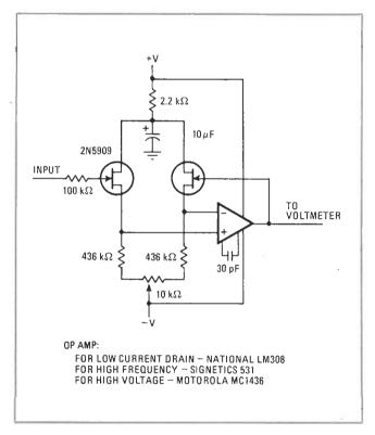
since FET gate-leakage current is in the low-picoampere range, the resistors used for the voltage divider can have values that are quite large without introducing significant errors. For example, a 1,000-megohm resistor to ground, along with another resistor having the appropriate value to obtain the desired ranging, will still provide an unusually high input resistance of several thousand megohms.
