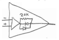
Most LM324 macro-models don't include the inherent output nonlinearity. Make a new model, as shown, with about two diodes added, and this makes a reasonable model. To defeat this non-linearity, add a pull-down resistor to the negative supply, making the output run Class A, for small signals.
