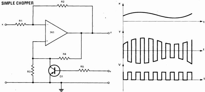
The circuit shown is a simple amplifier, the gain of which can be switched between two precisely controlled values by the application of a signal voltage: V. If V is such that Q1 is saturated, then the voltage gain of the circuit is simply  $\frac{R.2}{R.1}$ . If the transistor is cut off, then the voltage gain be-
