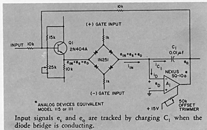
Input signals  $e_i$  and  $e_o$  are tracked by charging  $C_1$  when the diode bridge is conducting.
