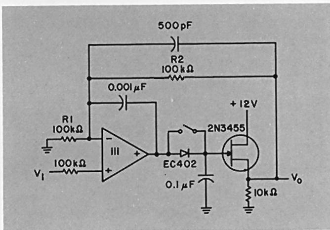
The illustrated circuit overcomes the above disadvantages, giving, for pulses of 2 to 300ms, an output that is not a function of pulselength and providing a linear  $V_0/V_1$  relationship. Performance was not investigated beyond these limits or for  $V_1$  greater than 4V. The graph shows the linearity and independence of pulselength that was achieved.
