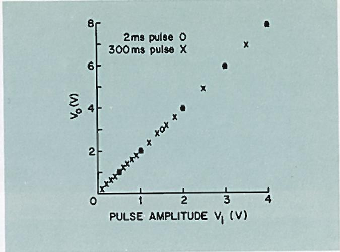
Analog 111, the diode is a low-reverse-leakage type and the field-effect transistor is by Amelco. The circuit will hold the peak value of an applied pulse for an hour or more if due attention is paid to insulation. Closing the switch resets the system to zero. A 20000 $\Omega$ /V meter was used to record  $V_0$ , but in the final application an emitter follower is connected to the field-effect transistor and the feedback loop taken from the emitter-follower output.
