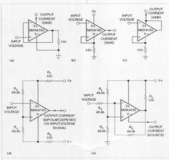
Figure 1 This compendium of constant-current circuits includes current sinks (a, b, and c), a bipolar sink or source (d), and a current source (e).
