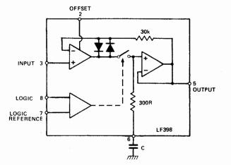
Use a printed circuit guard ring (connected to the output voltage) around the hold capacitor
