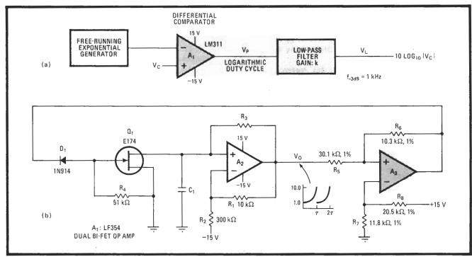
**Naturally.** Low-cost generator provides exponential waveform of sufficient accuracy in amplifier that takes logarithms over one decade of input voltage. Filter averages pulse-width-modulated equivalent of  $V_c$  produced by differential comparator,  $A_1$ , for  $V_L = 10 \log_{10} V_c$ .
