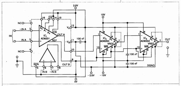
Figure 1 By cascading an autozeroed instrumentation amplifier having a gain of 2<sup>3</sup> and instrumentation amplifiers having gains of five, you get a decade-gain instrumentation amp whose dc performance is much better than that of monolithic decade-gain instrumentation amps.
