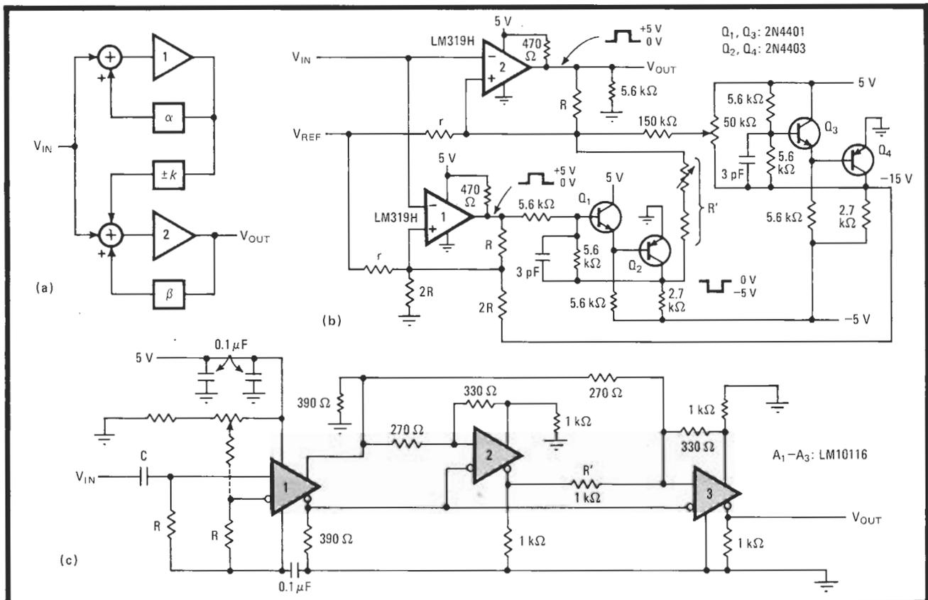
**Ideal.** Amplifiers with high loop gain work as nearly perfect comparators and zero-crossing detectors when they are suitably combined to cancel hysteresis (a). The implementation of a practical comparator (b) and a zero-crossing element (c) are relatively simple.
