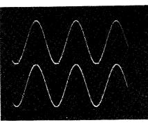
Lower trace is the input signal; upper trace is the output from the restorer. Oscillogram was obtained with the circuit operating on a 150Hz signal with an amplitude of 40mV peak-to-peak.
