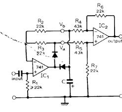
The required voltage waveform, with its minimum d.c. level restored to zero, appears as  $V_a - V_b$ . A low-impedance single-ended output is provided by IC, and, in this case, unity gain overall. Using a 250-µF electrolytic capacitor,
