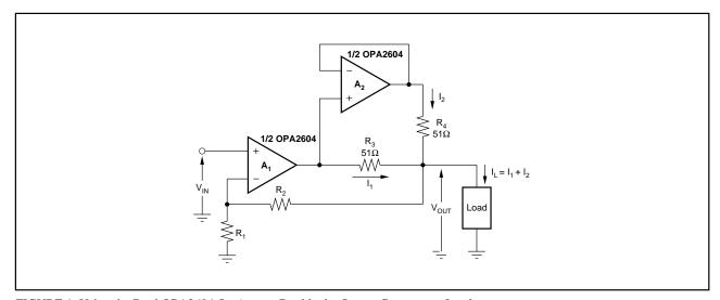
FIGURE 1. Using the Dual OPA2604 Op Amp to Double the Output Current to a Load.
