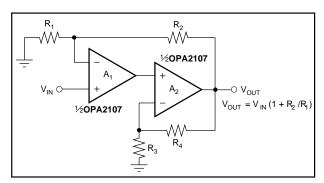
FIGURE 3. Composite Noninverting Amplifier Using Dual Op Amp Settles Fast.
