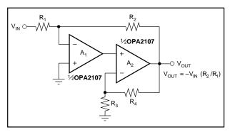
FIGURE 4. Composite Inverting Amplifier Using Dual Op Amp Settles Fast.
