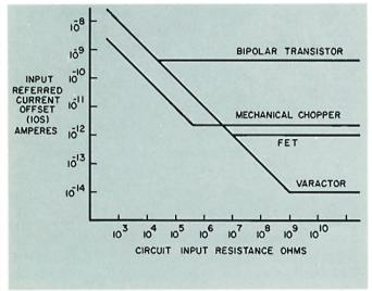
Notice that for integrator input resistance values of ten megohms or less, about equal performance can be expected from either a FET or a varactor amplifier. For input resistance values less than several megohms, best performance is offered by mechanical chopper amplifiers.
