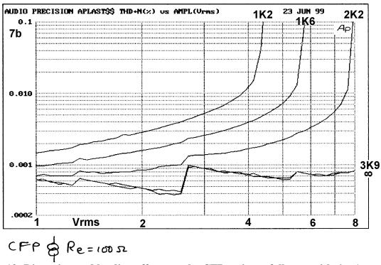
Fig 12: Distortion and loading effects on the CFP emitter-follower with 6 mA current-source. The steps on the lower traces are artefacts caused by the measurement system gain-ranging as it attempts to measure the THD of pure noise. (7B)
