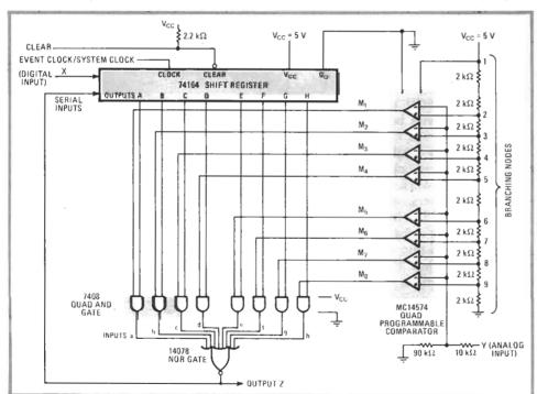
1. Variable counter. Using a voltage-divider network as the input to the MC14574 programmable comparator determines the analog levels necessary to create the control word that determines the divide-by-N action. The threshold at each mode differs by .5 V.
