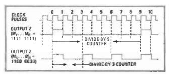
2. Divide-by-N waveforms. With the shift register initially cleared and a control word consisting of all 1s, the Z output of the NOR gate, in this case a logical 1, is fed to the shift register upon presence of a clock pulse. The Z output goes high every ninth clock pulse, providing divide-by-9 action.
