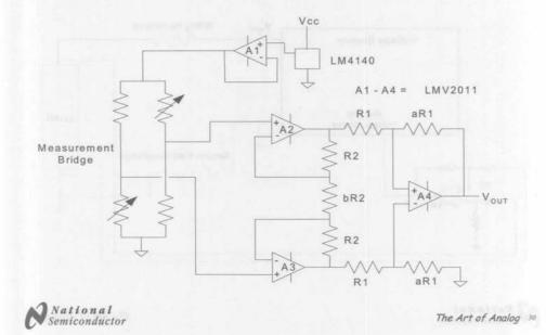
Bridge based transducers are used in a variety of measurement instruments. The signal level from Bridges are typically low level ranging from several hundred microvolts to a few millivolts. The excitation voltage must be stable since changes in the excitation voltage can be interpreted as a bridge measurement signal. The circuit shown here address both of these issues.
