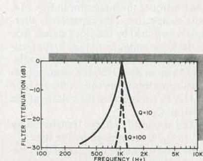
Fig. 15. Logarithmic plot of the same bandpass curve as shown in Fig. 14.
