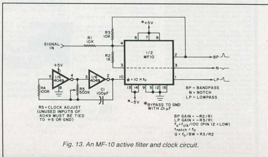
Fig. 13. An MF-10 active filter and clock circuit.
