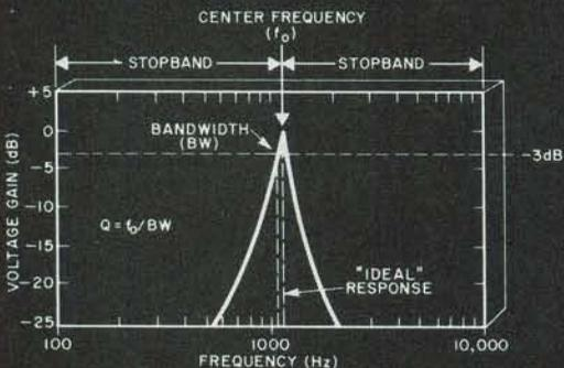
Fig. 10. Bandpass active filter characteristic.
