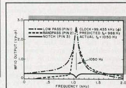
Fig. 14. Response of MF-10 (mode 1— at clock frequency of 99.435 kHz.
