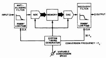
\* The R5609 has a rolloff slope of 100 dB/octave
