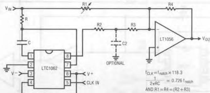
Figure 18. Using the LTC1062 to Create a Notch
