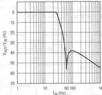
Figure 22. Amplitude Response of the Filter, Figure 21
