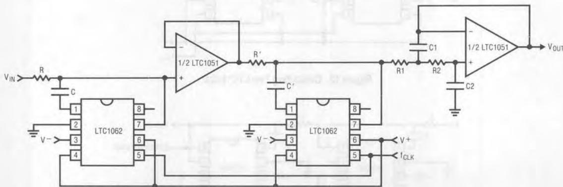
**Figure 15. A Very Low Offset, 12th Order, Max Flat Lowpass Filter**
