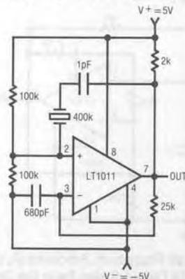
Figure 25. Crystal Oscillator with 50% Duty Cycle
