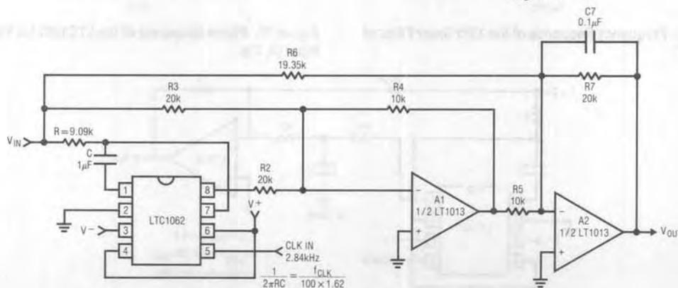
Figure 21. A Lowpass Filter with a 60Hz Notch
