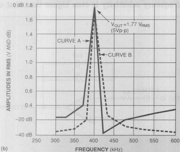
**Fig 1—One amplifier and a ceramic resonator create a bandpass filter (a). The solid curve of b shows the filter's frequency response. Note the dip to -40 dB on the high side of resonance. The dip is the result of the resonator's parasitic capacitance.**
