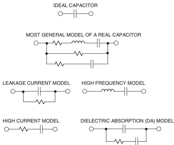
**Figure 5-83: Capacitor equivalent circuit**
