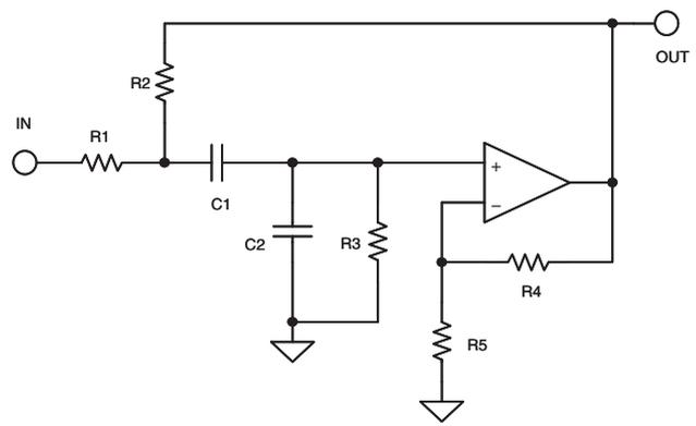
Figure 5-51: Sallen-Key band-pass filter
