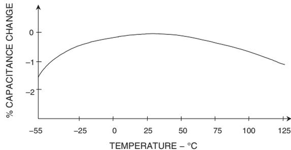
Figure 5-82: A poor film capacitor temperature coefficient
