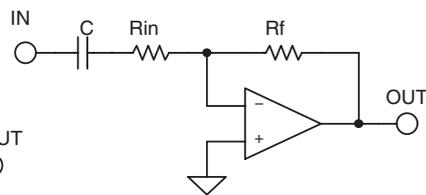
$$\frac{V_o}{V_{IN}} = -\frac{R_f}{R_{in}} \frac{sC R_1}{sC R_1 + 1}$$
