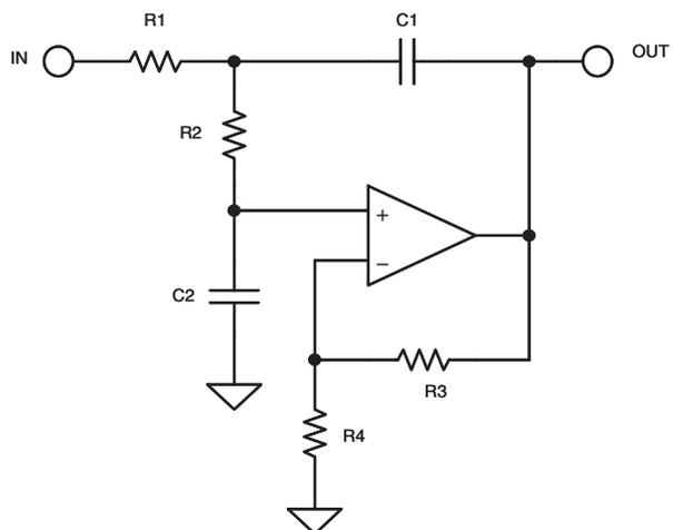
due to the fact that the op amp is configured as an amplifier, as opposed to an integrator, which minimizes the gain-bandwidth requirements of the op amp. This infers that for a given op amp, it is possible to design a higher frequency filter than with other topologies since the op amp gain bandwidth product will not limit the performance of the filter as it would if it were configured as an integrator. The signal phase through the filter is maintained (noninverting configuration).
