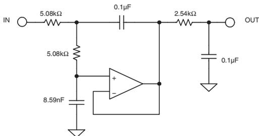
Using the equation string described in Section 5, the filter is now transformed into a high-pass filter. The results of the transformation are:
