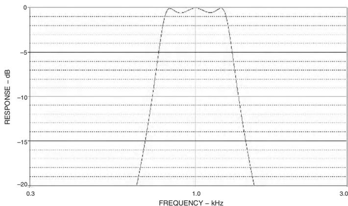
Note that again there is symmetry around the center frequency. Also the 500 Hz bandwidth is not 250 Hz either side of the center frequency (arithmetic symmetry). Instead the symmetry is geometric, which means that for any two frequencies ( $F_1$  and  $F_2$ ) of equal amplitude are related by:
