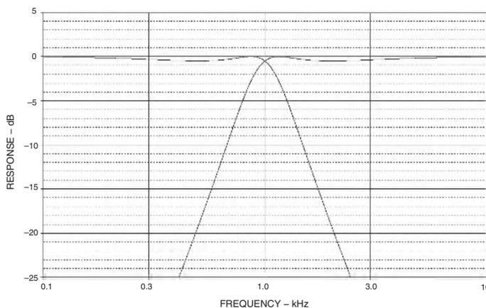
Part of the transformation process is to specify the 3 dB bandwidth of the resultant filter. In this case this bandwidth will be set to 500 Hz. The results of the transformation yield:
