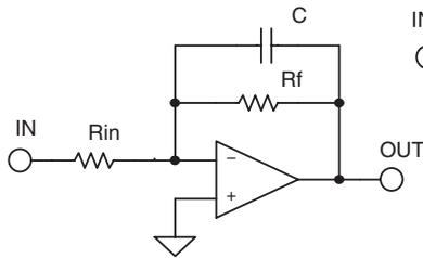
$$\frac{V_o}{V_{IN}} = -\frac{R_f}{R_{in}} \frac{1}{sC R_2 + 1}$$
