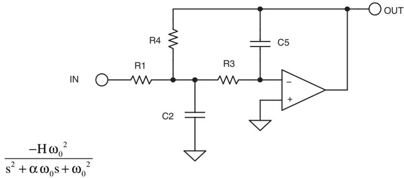
$$\frac{V_O}{V_{IN}} = \frac{-H \frac{1}{R_3 R_4 C_2 C_5}}{s^2 + s \frac{1}{C_2} \left( \frac{1}{R_1} + \frac{1}{R_3} + \frac{1}{R_4} \right) + \frac{1}{R_3 R_4 C_2 C_5}}$$
