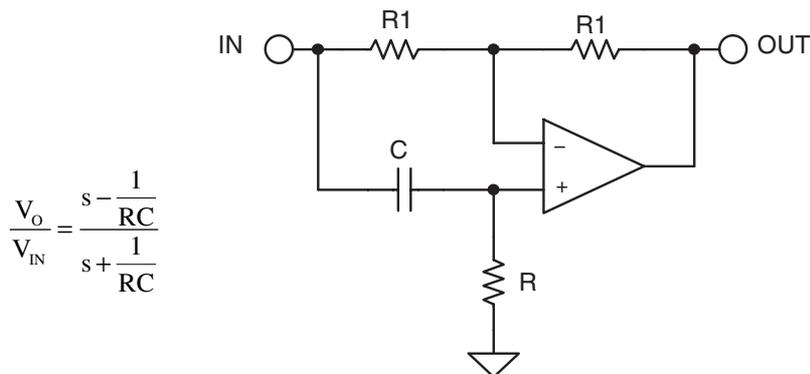
$$\frac{V_o}{V_{IN}} = \frac{s - \frac{1}{RC}}{s + \frac{1}{RC}}$$
