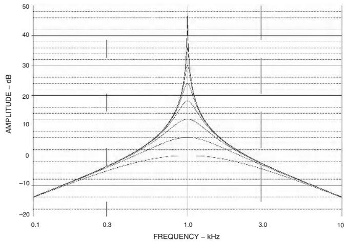
Figure 5-115: Gain variation versus DAC control word
