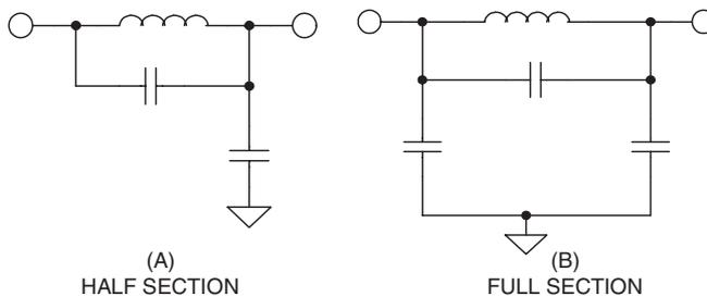
Figure 5-40: Passive filter blocks (low pass m-derived)
