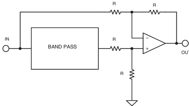
Figure 5-63: 1 – BP filter for noninverting band pass configurations
