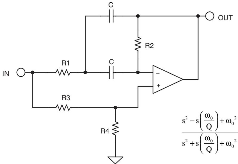
$$\frac{s^2 - s\left(\frac{\omega_0}{Q}\right) + \omega_0^2}{s^2 + s\left(\frac{\omega_0}{Q}\right) + \omega_0^2}$$
