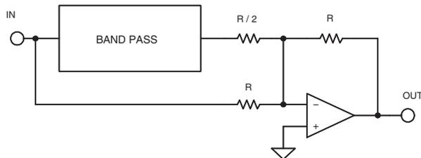
Figure 5-62: 1 – BP filter for inverting band pass configurations
