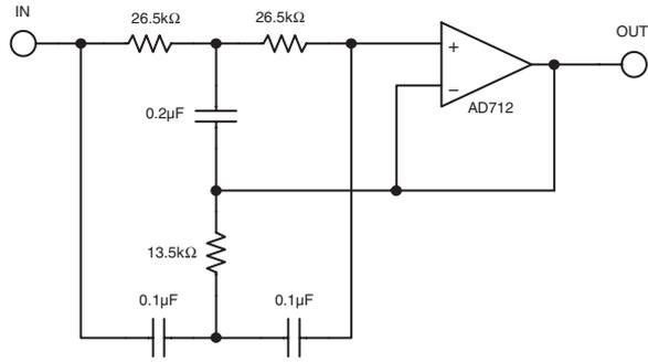
Figure 5-117: 60 Hz Twin-T notch filter
