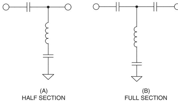
Figure 5-42: Passive filter blocks (high pass m-derived)
