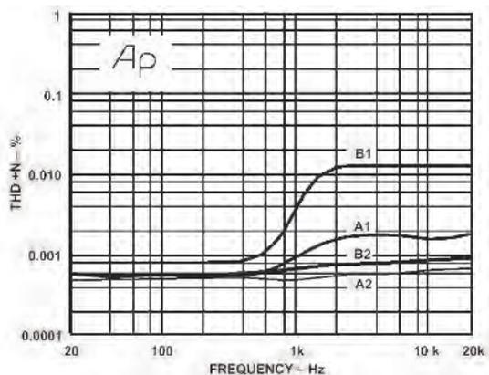
Figure 5-87: Distortion due to input capacitance modulation
