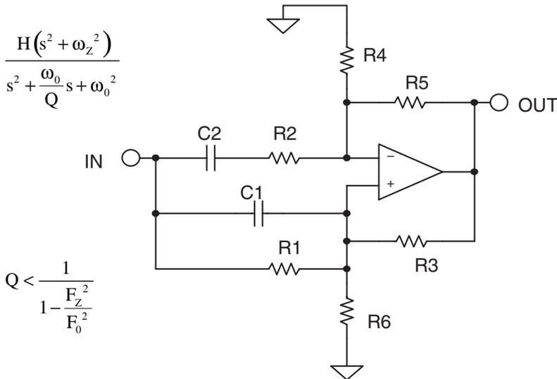
$$\frac{V_{OUT}}{V_{IN}} = \frac{\left(1 + \frac{R5}{R4}\right) \left(s^2 + \frac{1}{R1 R2 C1 C2}\right)}{s^2 \left[ \frac{1}{R_{EQ1} C1} \left(1 - \frac{R_{EQ1} R_{EQ2}}{R1 R2}\right) \right] s + \frac{1}{R_{EQ1} R_{EQ2} C1 C2}}$$
