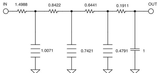
Figure 5-109C: CD Reconstruction filter—normalized FDNR
