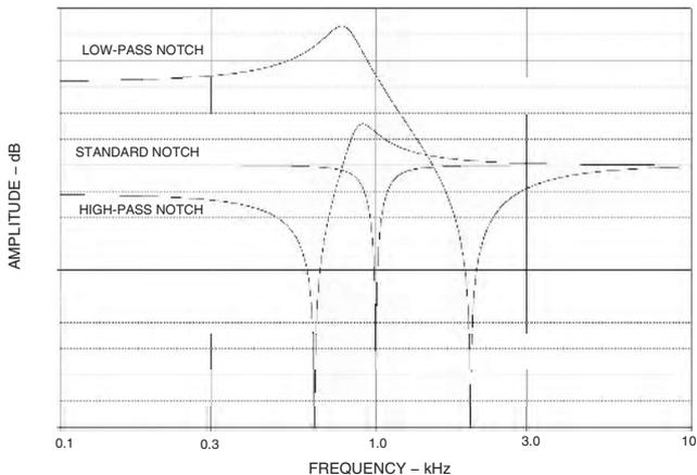
If the zero frequency is equal to the pole frequency a standard notch exists. In this instance the zero lies on the  $j\omega$  plane where the curve that defines the pole frequency intersects the axis.
