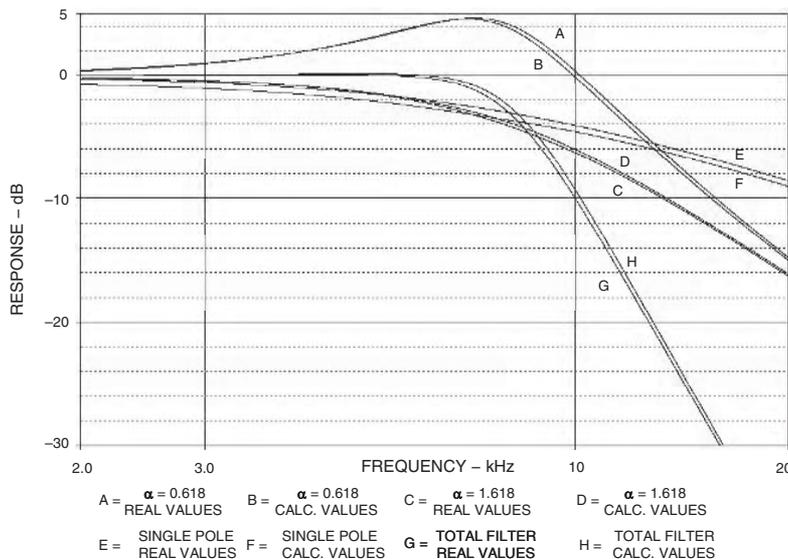
Figure 5-100: Effect of using standard value resistors
