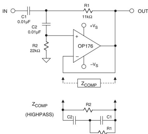
Figure 5-86: Compensation for input capacitance voltage modulation
