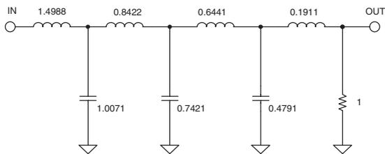
Figure 5-109B: CD Reconstruction filter—transformation in  $s$ -plane
