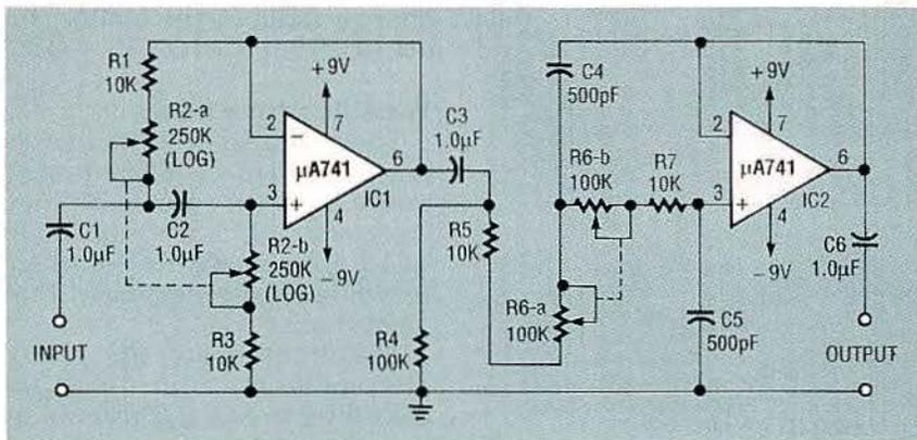
FIG. 12—A VARIABLE HIGH-PASS/LOW-PASS OR RUMBLE/SCRATCH audio filter.
