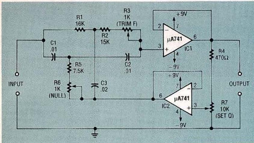
FIG. 16—A VARIABLE-Q, BOOTSTRAPPED TWIN-T NOTCH filter for 1 kHz.
