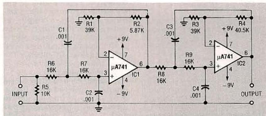
FIG. 5—A FOURTH-ORDER LOW-PASS FILTER for 10-kHz signals.
