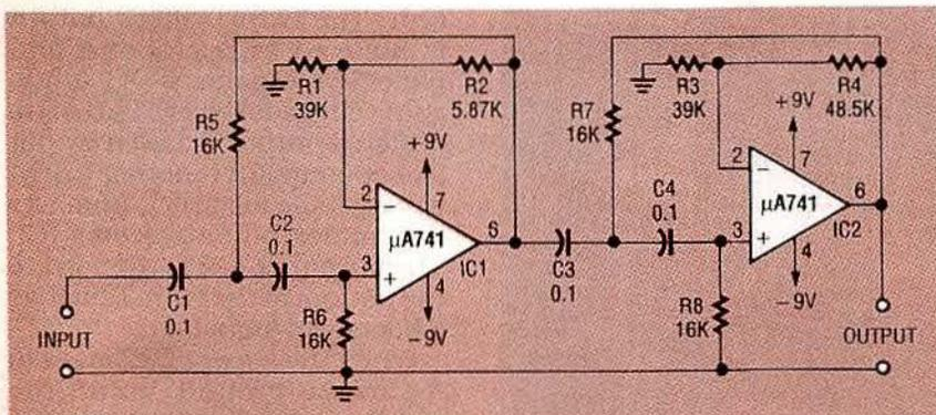
FIG. 8—A FOURTH-ORDER HIGH-PASS FILTER for 100-Hz signals.
