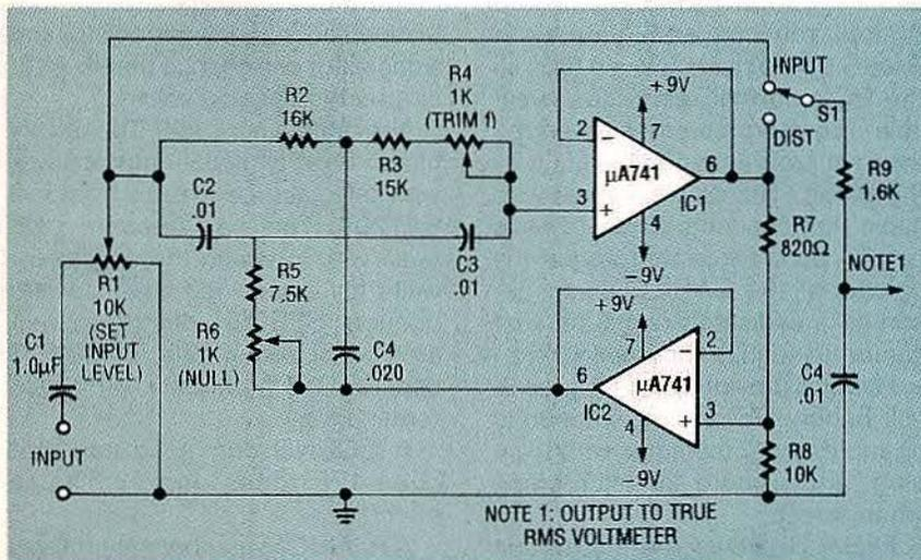
FIG. 17—THE SCHEMATIC FOR A 1-kHz TOTAL HARMONIC DISTORTION (THD) meter circuit.
