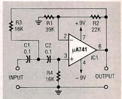
FIG. 7—AN EQUAL COMPONENTS second-order 100-Hz high-pass filter.
