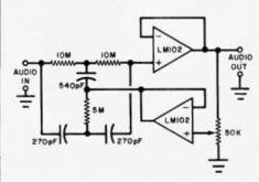
output of the second voltage follower for the twin-T R-C filter permits varying Q from 0.3 to 50. This varies the width of the 60-Hz notch. The notch depth depends on component matching. Using 1% resistors and 1% capacitors should give good results.
