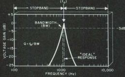
Fig. 10. Bandpass active filter characteristic.
