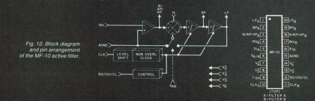
filters, each of which performs five basic filter functions (lowpass, highpass, bandpass, notch and allpass) with only a few external resistors and no external capacitors—well, almost no capacitors. Unlike conventional active filters, the MF-10 requires an input clock, and clock circuits usually incorporate a capacitor or two. The clock capacitor poses no tolerance problem, however, since the clock's frequency can be easily tuned by changing the value of a single resistor.
