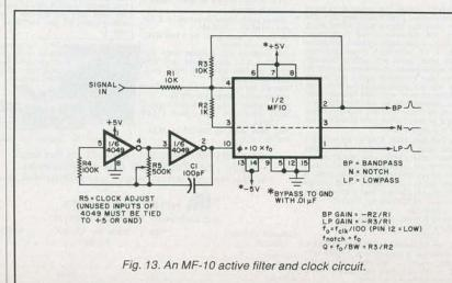
$f_{\rm o})$ , and the BP/notch Q is 10. The circuit can easily be tuned out to a maximum  $f_{\rm o}$  of 30 kHz simply by altering the clock frequency (where the ratio of clock frequency-to- $f_{\rm o}$  is approximately 100:1). The gain and Q values can easily be altered by changing the resistors.
