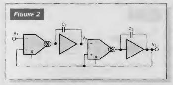
Adding integrating amplifiers reduces the effect of the multiplier capacitance, allowing a higher cutoff frequency. Note the reversed multiplier input connections. The transfer function is the same as in Figure 1.
