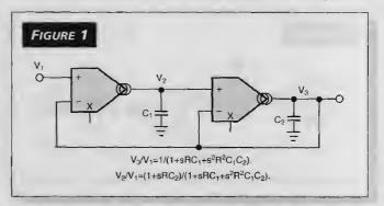
This Sallen-Key filter is implemented with current-output multipliers, where R is the multipliers' voltage-controlled transimpedance.
