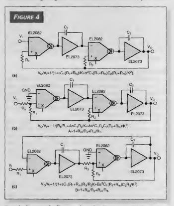
Practical two-pole filters using the Elantec multiplier show some of the possible implementations for this topology. The filter in (a) has high input impedance and can be driven from any source; however, it shows more high-frequency feedthrough than (b) and (c).
