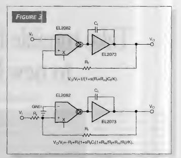
Single-pole filters using an Elantec EL2082 multiplier offer an alternative topology. K is the multiplier's current gain;  $R_m$  is its input resistance, about 95 $\Omega$ .
