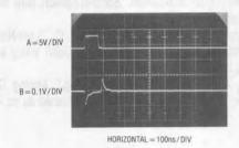
Figure B6. Response of  $10\mu F$  Aluminum Paralleled by  $0.01\mu F$  Ceramic
