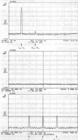
Figure 23. Elliptic Switched Capacitor Filter (LTC1064-1) Aliasing Study.  $f_0 = 500$ Hz,  $f_{CLK} = 50$ kHz,  $V_{S} = \pm 8V$ ,  $V_{IN} = 49.9$ kHz @ 500m $V_{RMS}$ . Note Dynamic Range Limitation.
