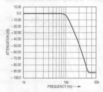
Figure 32. Frequency Domain Response of LTC1064-2 Butterworth Filter.  $f_{CUTOFF}$  = 10kHz,  $V_{S}$  =  $\pm$  7.5V, LT1007 Output Buffer, 50:1.
