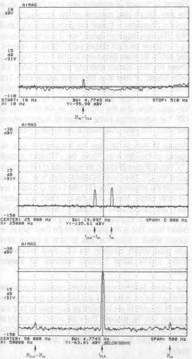
Figure 22. Elliptic Switched Capacitor Filter (LTC1064-1) Aliasing Study.  $f_0 = 500$ Hz,  $f_{CLK} = 50$ kHz,  $V_S = \pm 8V$ ,  $V_{IN} = 25.1$ kHz @ 500mV<sub>RMS</sub>.
