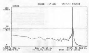
Figure 9. Wideband Noise Measurement — 8th Order Elliptic Lowpass Filter (LTC1064-1) Using Good Breadboarding Techniques.  $f_{CLK}$  = 2MHz,  $f_{CUTOFF}$  = 20kHz,  $V_S$  =  $\pm$  8V, Buffered with LT1007.
