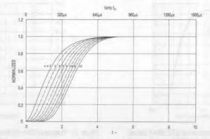
Figure 28. Step Response for Synchronously Tuned Filters\*
