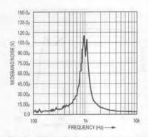
Figure 46. Noise Spectrum of Bessel BPF as Shown in Figure 43. Input Grounded. Total Wideband Noise =  $130\mu V_{RMS}$ .
