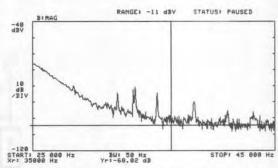
Figure 10. Stopband Response — 8th Order Elliptic Lowpass Filter (LTC1064-1). Power Supply Is Unbypassed Industry Standard Modular +5V to  $\pm15V$  Switcher. The Improperly Constructed Breadboard Was Used For This Test.  $f_{CLK}=2MHz$ ,  $f_{CUTOFF}=20kHz$ ,  $V_S=\pm7.5V$ , (Switcher Zenered to  $\pm7.5V$ ).
