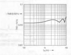
Figure 38. LTC1064-2 THD + Noise vs Input Frequency. Filter  $f_{CUTOFF} = 8kHz$ ,  $f_{CLK} = 800kHz$ ,  $V_S = \pm 5V$ ,  $V_{IN} = 1.5V_{RMS}$ , Buffered Output Using LT1006.
