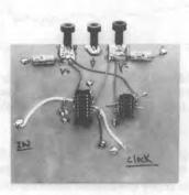
Figure 5. Properly Constructed "Good" Switched Capacitor Filter Breadboard
