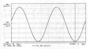
Figure 17. Small Signal Response — Output of Elliptic Filter (LTC1064-1) Plus Servo (Figure 14). Input: 50mV<sub>RMS</sub>, 2Hz Sine Wave. Filter f<sub>CUTOFF</sub> = 100Hz.
