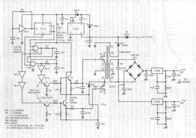
Figure 11. Low Noise 5V to ±7.5V Converter (200μVp-p Noise)
