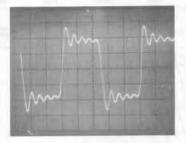
Figure 29. LTC1064-1 Time Domain Response. Filter fcuToFF = 100Hz. Input: 10Hz Square Wave. Horiz = 20ms/Div., Vert = 0.5V/Div.
