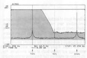
Figure 61. Frequency Domain (Spectrum Analyzer) Plot of 7500Hz Square Wave (5Vp-p) *Input* to LTC1064-1 as Configured in Figure 4. fcutoff = 10kHz. *Shaded Area* is the Frequency Response of the Filter.
