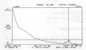
Figure 8. Wideband Noise Measurement — 8th Order Elliptic Lowpass Filter (LTC1064-1) Using Improper Breadboarding Techniques.  $f_{CLK} = 2MHz$ ,  $f_{CUTOFF} = 20kHz$ ,  $V_S = \pm 8V$ , Buffered with LT1007.
