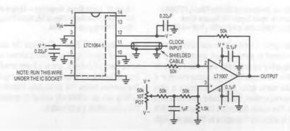
Figure 12. Elliptic Filter with Offset Adjustment Potentiometer
