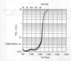
Figure 40. LTC1064-2 THD + Noise vs Input Amplitude and Signal to Noise Ratio. Filter  $f_{CUTOFF} = 8kHz$ ,  $f_{CLK} = 800kHz$ ,  $f_{IN} = 1kHz$ ,  $V_S = \pm 5V$ , Inverting Buffer Using LT1006. Four Devices Superimposed.
