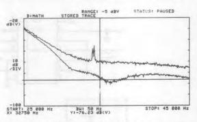
Figure 7. Stopband Response — 8th Order Elliptic Lowpass Filter (LTC1064-1). Top Trace: Improperly Constructed Breadboard, No Buffer. Bottom Trace: Good Breadboard, with Buffer. Both: fcl K = 2MHz, fcutoff = 20kHz, Vs = ±8V.
