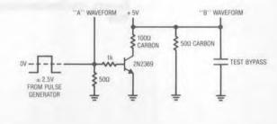
Figure B2. Bypass Capacitor Test Circuit
