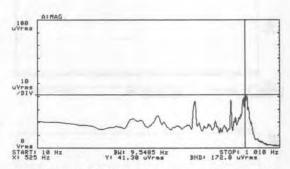
Figure 49. Noise of LTC1064-1 as per Figure 48 with  $\approx$  50% Clock Jitter.  $V_S = \pm 7.5V$ , Input Grounded.
