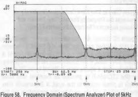
Figure 58. Frequency Domain (Spectrum Analyzer) Plot of 5kHz Square Wave (5Vp-p) *Input* to LTC1064-1 as Configured in Figure 4. fcutoff = 10kHz. *Shaded Area* is the Frequency Response of the Filter.
