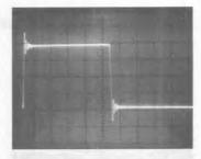
Figure 13. Time Domain Response of Elliptic Filter (LTC1064-1) Without Servo in Figure 12. Input Signal 1Hz Square Wave. LTC1064-1 Cutoff (f<sub>o</sub>) = 100Hz. Horiz = 0.1s/Div., Vert = 0.5V/Div.
