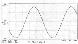
Figure 18. Input Signal (50mV<sub>RMS</sub>, 0.092Hz) to Elliptic Filter (LTC1064-1) as Shown in Figure 14.
