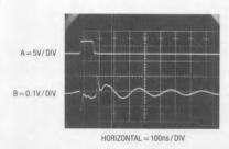
Figure B7. Some Paralleled Combinations Can Ring. Try Before Specifying!
