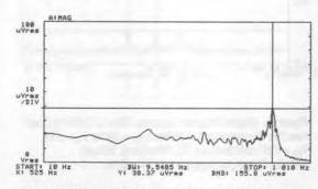
Figure 50. Noise of LTC1064-1 as per Figure 48 with Low Jitter (<1ns).  $V_S = \pm 7.5V$ , Input Grounded.
