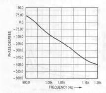
Figure 47. Passband Phase Response of Bessel BPF as Shown in Figure 43. Note the Linear Phase Through the Passband.
