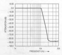
Figure 34. Frequency Domain Response of LTC1064-4 Elliptic Filter.  $f_{CUTOFF} = 10kHz$ ,  $V_S = \pm 7.5V$ , LT1007 Output Buffer, 50:1.
