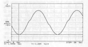
Figure 16. Large Signal Response — Output of Elliptic Filter (LTC1064-1) Plus Servo (Figure 14). Input: 1V<sub>RMS</sub>, 0.092Hz Sine Wave. Filter f<sub>CUTOFF</sub> = 100Hz.
