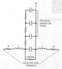
Figure B1. Parasitic Terms of a Capacitor
