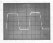
Figure 30. LTC1064-3 Time Domain Response. Filter fCUTOFF = 100Hz. Input: 10Hz Square Wave. Horiz = 20ms/Div., Vert = 0.5V/Div.
