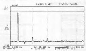
Figure 39. LTC1064-2 Spectrum Analyzer Plot for  $V_{IN}$  = 1.5 $V_{RMS}$ ,  $f_{IN}$  = 2kHz,  $V_{S}$  = ±5 $V_{S}$ , Buffered Output Using LT1006
