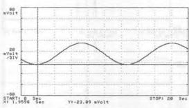
Figure 19. Small Signal Output Response of Elliptic Filter (LTC1064-1) Plus Servo to Input Shown as Figure 18. Filter fcutoff = 100Hz.
