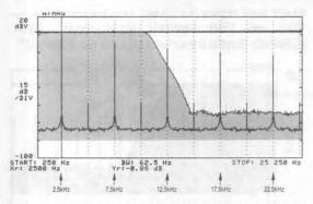
Figure 55. Frequency Domain (Spectrum Analyzer) Plot of 2500Hz Square Wave (5Vp-p) *Input* to LTC1064-1 as Configured in Figure 4. fCUTOFF = 10kHz. *Shaded Area* is the Frequency Response of the Filter.
