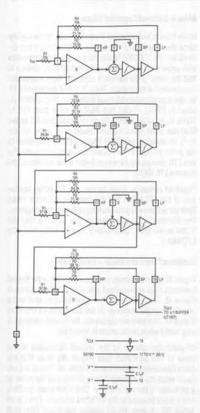
Figure 45. Implementation, Section by Section, of Bessel BPF as per Figure 43 Using LTC1064. For f<sub>CUTOFF</sub> = 1kHz, f<sub>CLK</sub> = 50kHz.
