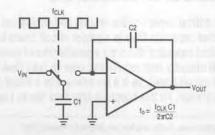
Figure 2. Inverting Switched Capacitor Integrator
