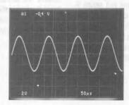
Figure 63. Filter Time Domain Output for Input 7.5kHz Square
