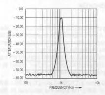
Figure 44. 8th Order Bessel Using LTC1064. V<sub>S</sub> = ±8V, V<sub>IN</sub> = 1V<sub>RMS</sub>, f<sub>CLK</sub> = 50kHz, f<sub>CUTOFF</sub> = 1kHz, Buffered Output.
