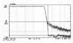
Figure 48. Clock Jitter of Approximately 50% (Top Curve in Stopband) and Jitter Free Clock (Bottom Curve in Stopband) Showing the Difference in Response. LTC1064-1, f<sub>CLK</sub> = 50kHz, f<sub>n</sub> = 500Hz, Buffered Output.
