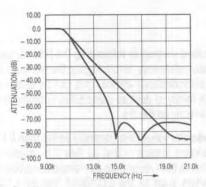
Figure 35. Frequency Domain Response of LTC1064-1 and LTC1064-4 Transition Region Blow-Up.  $f_{CUTOFF} = 10kHz$ ,  $V_S = \pm 7.5V$ , LT1007 Output Buffer.
