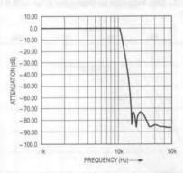
Figure 31. Frequency Domain Response of LTC1064-1 Elliptic Filter. f<sub>CUTOFF</sub> = 10kHz, V<sub>S</sub> = ±7.5V, LT1007 Output Buffer, 100:1.
