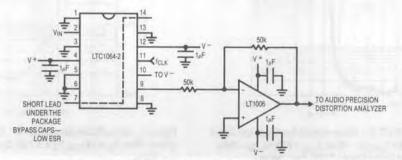
Figure 37. LTC1064-2 Circuit Used for THD Testing, Vs = ±5V.
