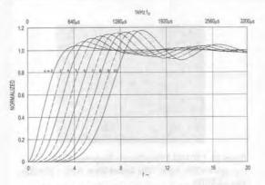
Figure 24. Step Response for Butterworth Filters\*
