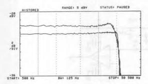
Figure 6. Passband Response — 8th Order Elliptic Lowpass Filter (LTC1064-1). Top Trace: Improperly Constructed Breadboard, No Buffer. Bottom Trace: Good Breadboard, with Buffer. Both:  $f_{CLK} = 2 \text{MHz}, f_{CUTOFF} = 20 \text{kHz}, V_S = \pm 8 \text{V. Note: Top Trace Was Offset to Increase Clarity.}$
