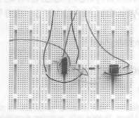
Figure 3. Improperly Constructed "Poor" Switched Capacitor Filter Breadboard
