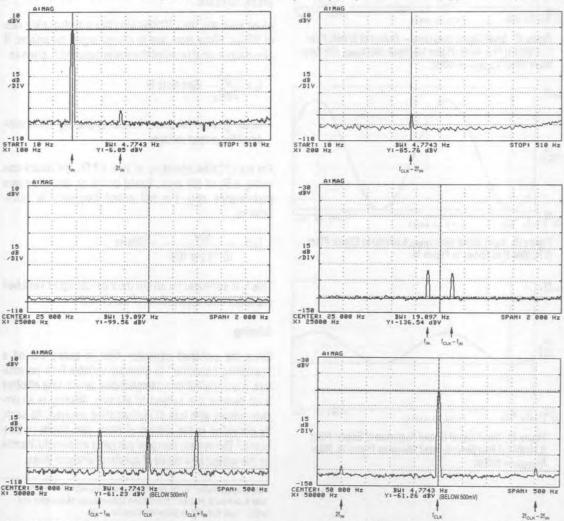
Figure 20. Elliptic Switched Capacitor Filter (LTC1064-1) Aliasing Study.  $f_0 = 500$ Hz,  $f_{CLK} = 50$ kHz,  $V_S = \pm 8V$ ,  $V_{IN} = 100$ Hz @ 500mV  $V_{RMS}$ . Note Dynamic Range Limitation.
