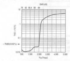
Figure 36. LTC1064-2 THD + Noise vs Input Amplitude and Signal to Noise Ratio. Filter  $f_{CUTOFF}$  = 8kHz,  $f_{IN}$  = 4kHz,  $f_{CLK}$  = 800kHz,  $V_S$  =  $\pm$ 5V. Inverting Buffer LT1006.
