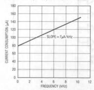
Figure 18. Current Consumption vs. Frequency for Figure 16
