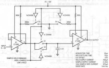
Figure 14. Micropower Sample-Hold
