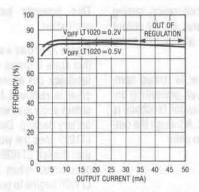
Figure 27. Figure 25's Efficiency vs. Output Current
