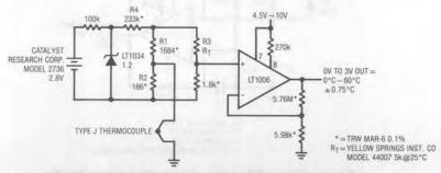
Figure 2. Thermocouple Signal Conditioner with Cold Junction Compensation
