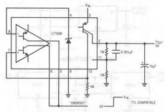
Figure 28. Regulator with Logic Output on Dropout
