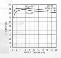
Figure 24. Figure 22's Efficiency vs. Output Current
