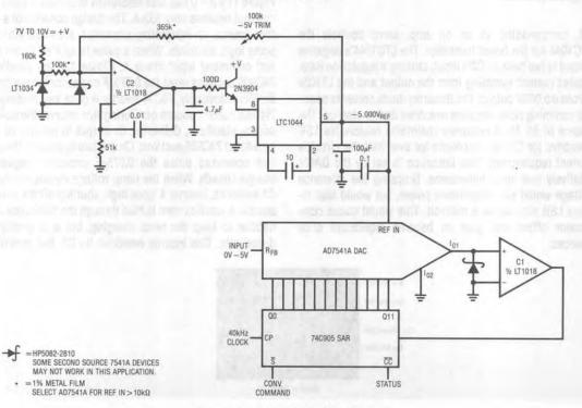
Figure 9. Micropower 12-Bit, 300µs A-D
