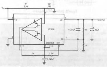
Figure 29. Regulator with Output Shutdown on Dropout
