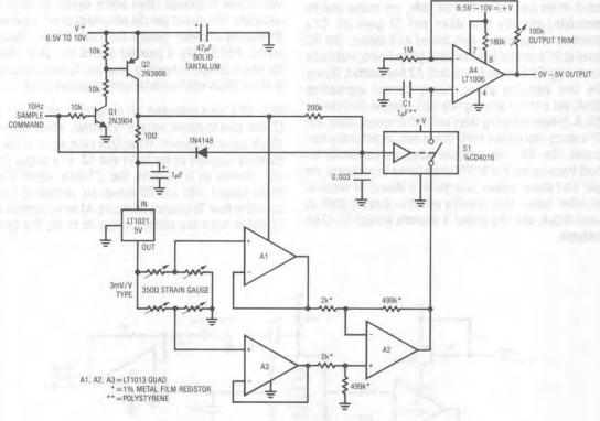
Figure 3. Sampled Strain Gauge Bridge Signal Conditioner
