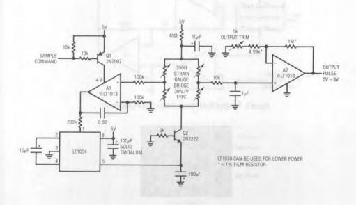
Figure 5. Strobed Power Strain Bridge Signal Conditioner
