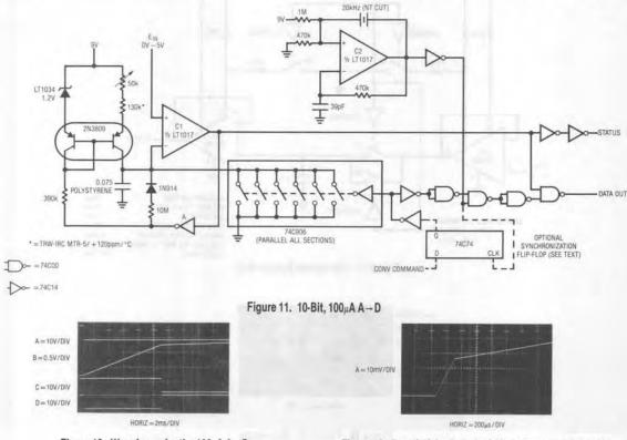
Figure 12. Waveforms for the 100µA A - D
