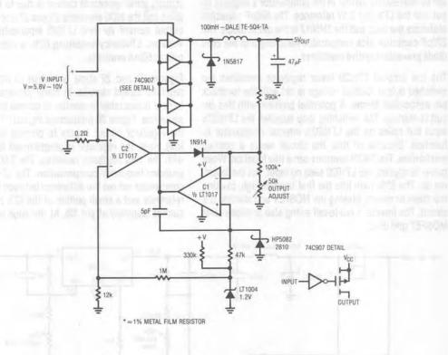
Figure 22. Micropower Switching Regulator
