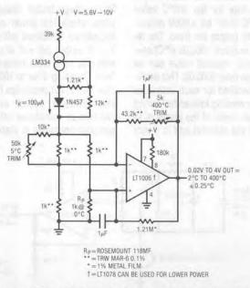
Figure 1. Platinum RTD Signal Conditioner with Curvature Correction
