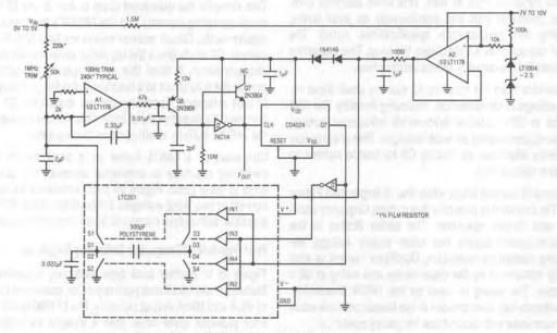
Figure 20. Micropower 1MHz V - F Converter
