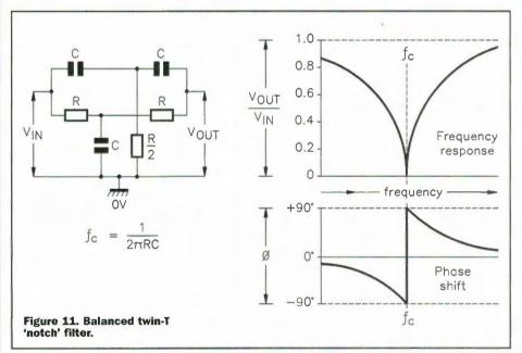
phase shifts of -45° and +45° respectively at fc simultaneously, the impedances of the R and C sections of the output divider are identical, and give a 45° phase shift at fc. Consequently, the divider effectively cancels the two phase differences under this condition and gives an output of precisely zero, this being the phase-cancelled difference in amplitudes of the two signals.
