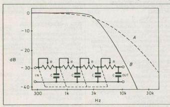
Fig. 1. Four-section RC low-pass network. Curve A shows the response of the network alone for values of R and C which produce a -3dB point at 3kHz. Curve B is for an active filter with a similar net-
