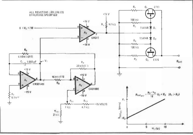
Ohmic linearization. FET switches in voltage controlled resistor network place maximum-minimum resistors R, and R, across Resistor that the resistance is proportional to the average time each is across output port, Switching technique ensures piecewise-linear operation. This circuit lends itself to many applications, such as a-m modulator, by placing voltage-controlled current source across Radio
