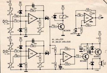
Using a single LM324 quad op-amp IC a versatile threshold comparator may be constructed. The circuit will sound an alarm and/or energise a relay whenever the input voltage falls outside preset levels. The circuit may be adjusted to respond to the three following conditions.
