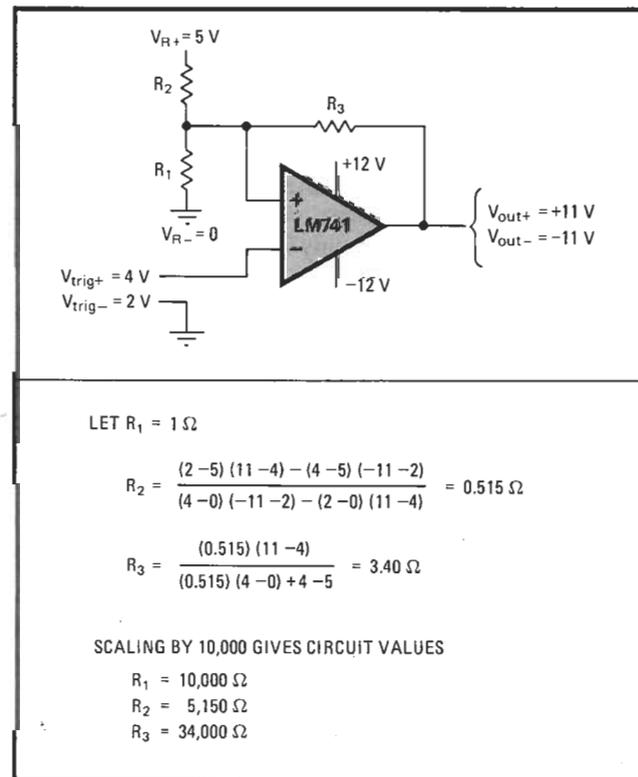
**2. Example.** Here is an inverting Schmitt circuit intended for trigger voltages of 2 and 4 V, output levels of  $\pm 11$  V, and a 5-V bias supply. The design equations yield resistance values that are then scaled up by 10,000 to match the National LM741 op amp, chosen because its  $\pm 12$ -V supply voltages bracket the desired output levels.
