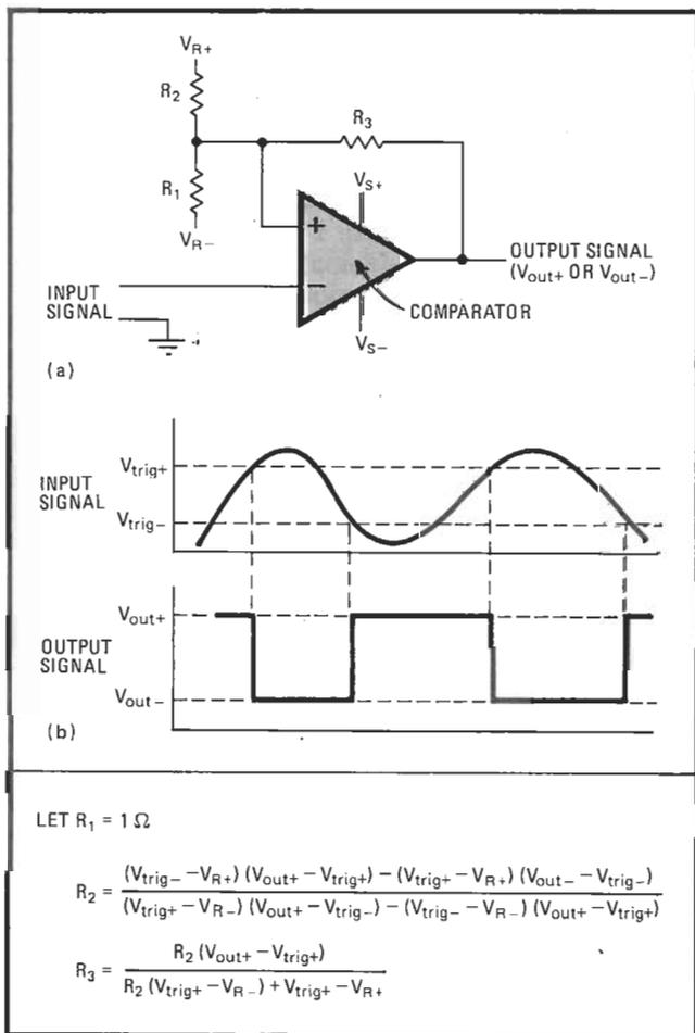
**1. Design equations.** Inverting Schmitt-trigger circuit (a) has triggering voltages and output levels as shown in (b). The circuit diagram and the waveforms illustrate the terms used in the design equations for resistors  $R_1$ ,  $R_2$ , and  $R_3$ . The resistance values found from these equations are then scaled up to match the comparator.
