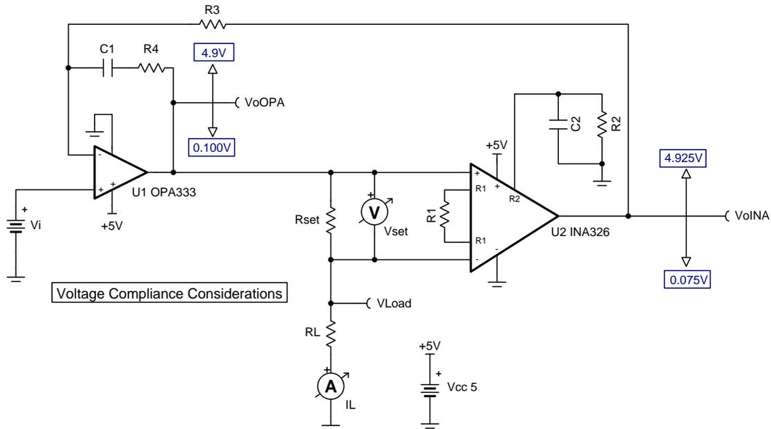
2. Compute instrumentation amplifier gain,  $G$ .
