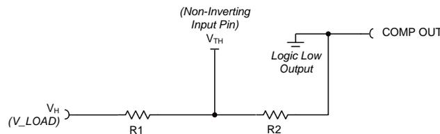
$$V_{TH} = V_H \times \left( \frac{R_2}{R_1 + R_2} \right)$$
