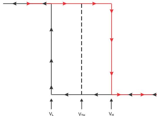
4. Derive the equation for  $V_H$ , which is the threshold voltage when  $V_o$  is high. For simplicity, assume  $V_o$  switches to  $V_{cc}$  when  $V_i < V_L$ . When this occurs,  $R_1$  and  $R_3$  are in parallel.
