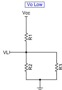
$$V_L = V_{cc} \times \frac{R_2 \parallel R_3}{R_1 + (R_2 \parallel R_3)}$$
