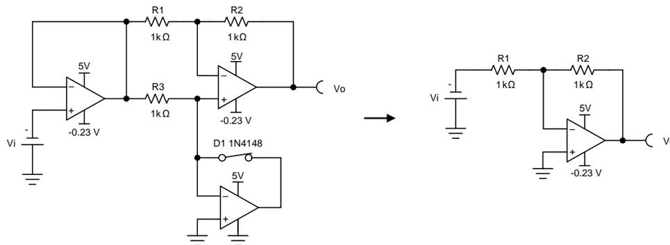
$$\frac{V_o}{V_i} = \left(-\frac{R_2}{R_1}\right) = -1$$
