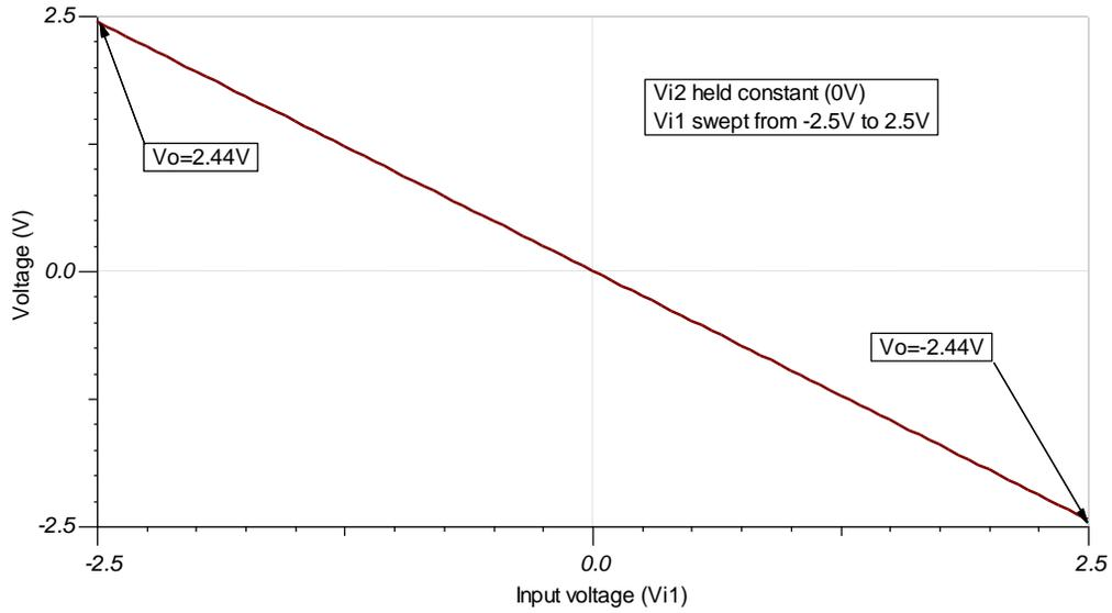
This simulation sweeps  $V_{i2}$  from  $-250mV$  to  $250mV$  while  $V_{i1}$  is held constant at  $0V$ . The output is inverted and ranges from  $-2.44V$  to  $2.44V$ .
