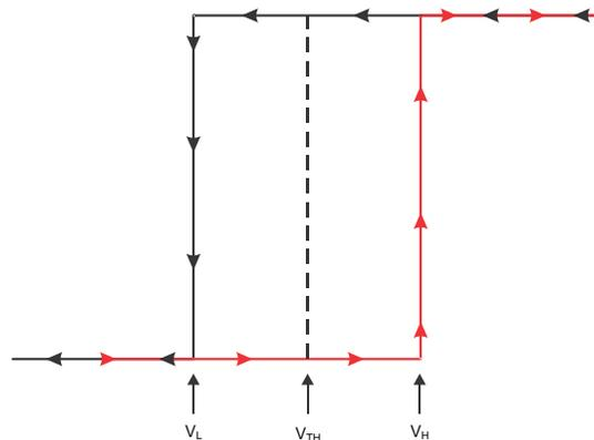
4. Derive the equation for  $V_H$ , the voltage that the input signal must rise to for the output to switch high. Set the voltage at the non-inverting pin to be equal to  $V_{TH}$ . This ensures the correct hysteresis window will be achieved.
