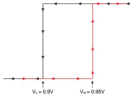
3. With the non-inverting input pin of the comparator labeled as  $V_{TH}$  and the comparator output in a logic low state (ground), derive an equation for  $V_{TH}$  where  $V_H$  represents the load voltage ( $V_{LOAD}$ ) when the comparator output transitions from low to high. Note that the simplified diagram for deriving the equation shows the comparator output as ground (logic low).
