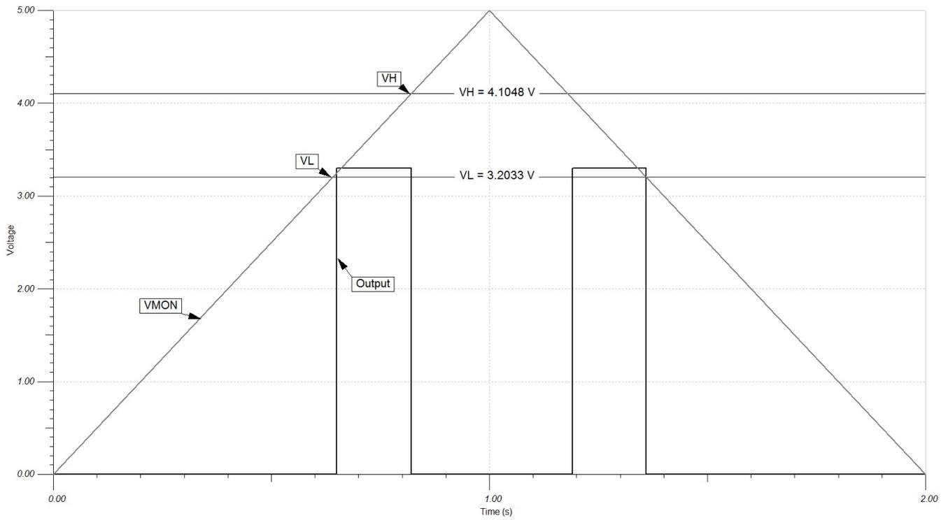
Note: The Rising edge  $V_L$  and falling edge  $V_H$  thresholds are slightly shifted due to the built-in asymmetrical hysteresis of the TLV6710. Comparators without hysteresis will meet the calculated thresholds.
