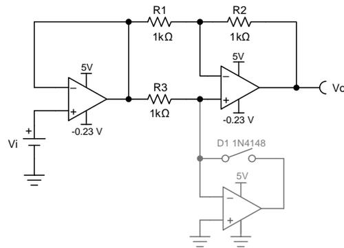
$$\frac{V_o}{V_i} = \left(-\frac{R_2}{R_1}\right) + \left(1 + \frac{R_2}{R_1}\right) = 1$$
