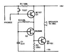
The disadvantage with battery operated alarm circuits is the quiescent current that they draw. The circuit shown above draws so little current that the shelf-life of the battery is the limiting factor - the only current drawn is the leakage of the transistors.
