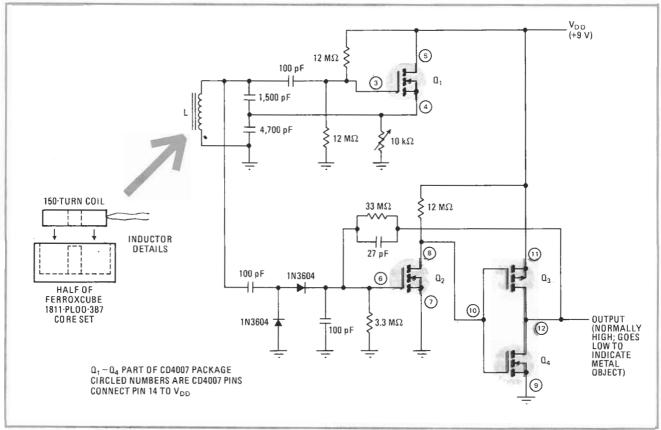
**Detects metal.** Proximity detector consists of modified Colpitts oscillator, amplitude detector, and Schmitt trigger. Output signal is normally high; but when oscillator coil is loaded by presence of metal object, amplitude decreases and output from Schmitt trigger goes low. Detail drawing shows construction of the oscillator coil in a proximity detector that serves as the noncontacting pickup for a tachometer.
