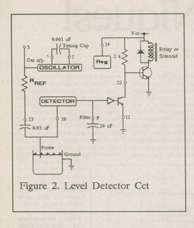
tor is no longer turned on. This constitutes an "active" low level indication, because the transistor is on when the level is below the electrode, but this can easily be inverted using another transistor (as shown in Figure 2) or by choosing the appropriate contact in the relay driven by the output.
