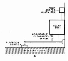
of a flotation device as shown in Fig. B), base current flows through Q1. The transistor then conducts and energizes relay K1. The relay contacts can be connected to an alarm, a pump, or any combination of devices.
