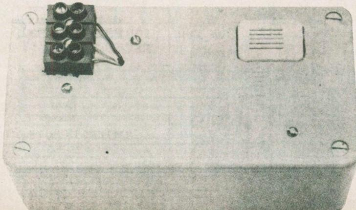
negative-ground car, connect the sensor wires to TB1/2 and TB1/3. Find a suitable fuse which is live only when the ignition is switched on and connect this to TB1/1. Make sure that the correct side has been used — when the fuse is removed the circuit should not work. Connect TB1/3 to an ground point (car chassis). For a positive-ground vehicle, make the sensor connections to TB1/2 and TB1/3. Connect the fuse to TB1/3 and TB1/1 to the ground point.
