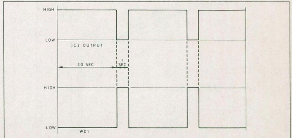
Fig. 2 IC2 output and WD1 drive waveforms.
