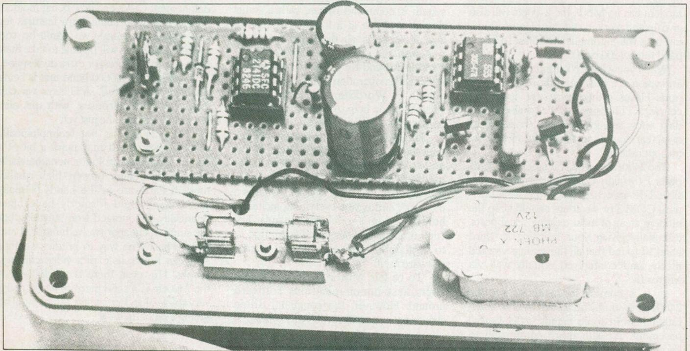
This circuit is designed to detect high temperatures, and has many uses; It could also be useful to readers who experience overheating problems with any car. It is suitable for both positive and negative ground systems.
