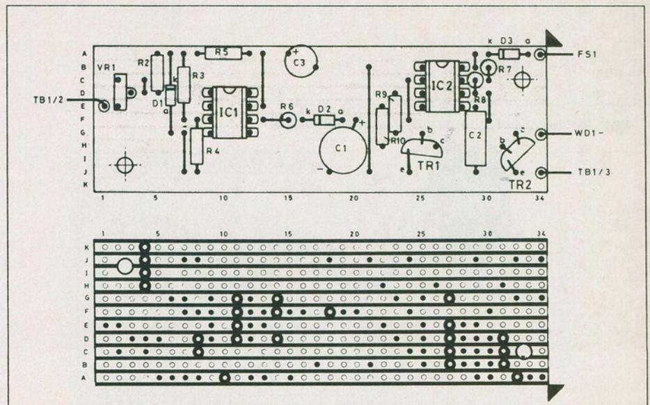
Fig. 3 Veroboard layout and wiring.
