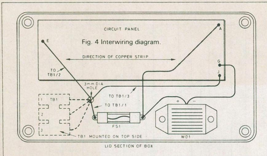
Fig. 4 Interwiring diagram.
