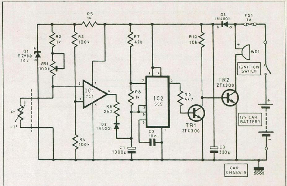
Fig. 1 Circuit diagram of the Thermal Alarm.
