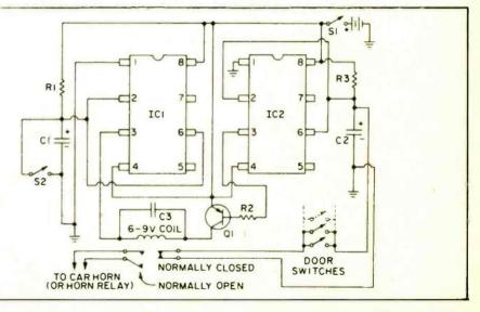
you to leave and enter the car without the horn will sound and will stay locked on until S1 is sounding. To set, or arm, the alarm circuit, open opened. If you open the door to enter, you have S2. This will give you five seconds (R1, C1) to get two seconds to close S2, which is plenty of time if out and shut the door behind you. If anyone S2 is conveniently located. opens a door for two seconds (R3, C2), the horn
