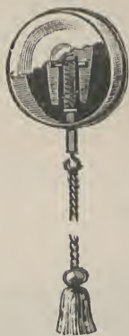
Fig. 18.—Electric Bell Pull.
