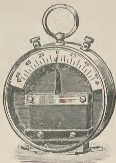
Fig. 26.—Pocket Galvanometer.
