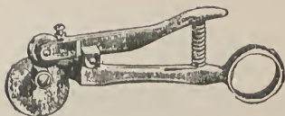
Fig. 58.—Tube Trimming Tool.
