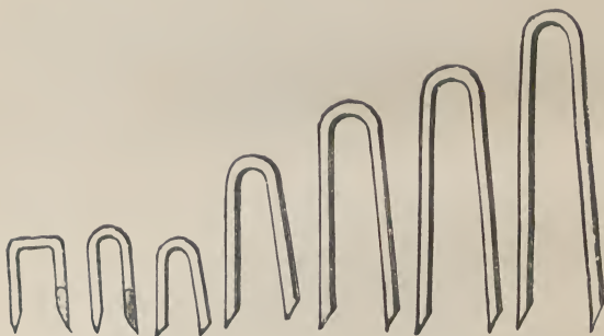
Fig. 4.—Staples for Securing Wires.
