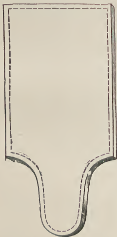
Fig. 87.—Wood Base-board of Electric Bell.
