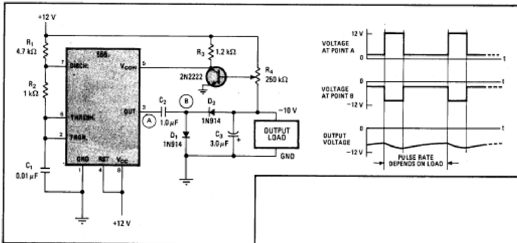
Latest addition to the 555 IC timer's seemingly endless bag of tricks is its use to generate a negative dc biasing voltage from a positive source. A current of well over 10 milliamperes can be delivered, and a form of switching regulation is employed to assure a constant output voltage. All of this is done with little more than an npn transistor and the 555 integrated circuit.
