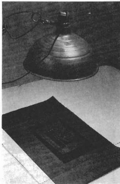
FIG. 3—A POSITIVE IMAGE is contact printed onto the stencil film using a photo flood bulb. Note the black paper beneath the film to prevent undercutting thin parts of the image.
