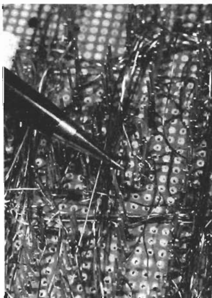
THE PENCIL POINTS to an area of wire-wrap pins that have bent over in their holes from handling. The posts themselves have not bent. Some of those posts will fall out of the holes when handled if the wire-wrapping hasn't been completed on them yet.
