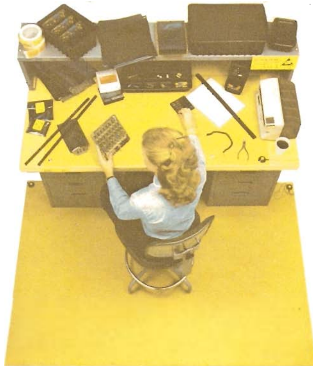
The static-safe work area is capable of controlling static charge on conductive objects, non-conductive objects and people
