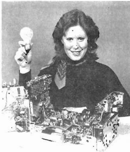
RCA's "XTENDED LIFE" CHASSIS uses only 89 watts to power the 19-inch models. This compares with the average solid-state color TV set that uses 145 watts.
